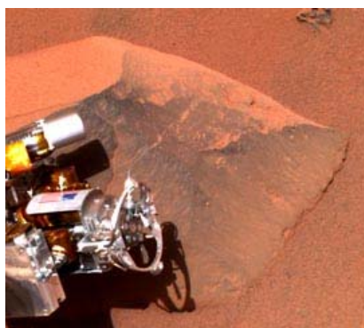
Spirit's robotic arm of tools before dusting off and grinding into the rock named "Adirondack" at the Gusev crater site.
