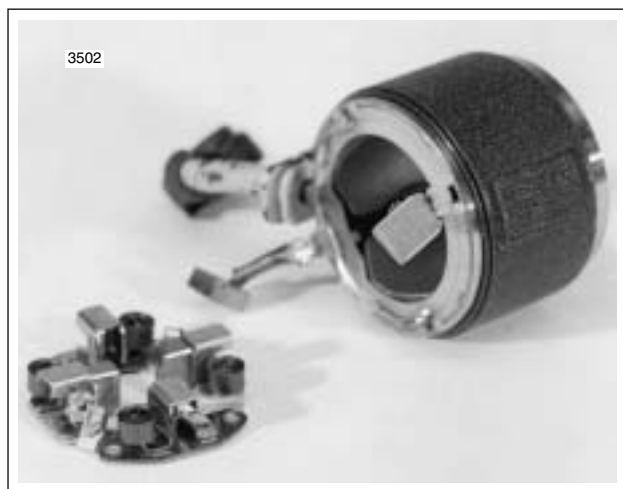
Figure 5-9. Remove Brush Holder
