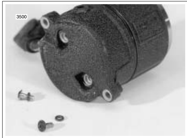
Figure 5-7. Remove End Cap Screws and O-Rings
