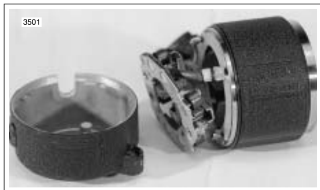
Figure 5-8. Remove End Cap
