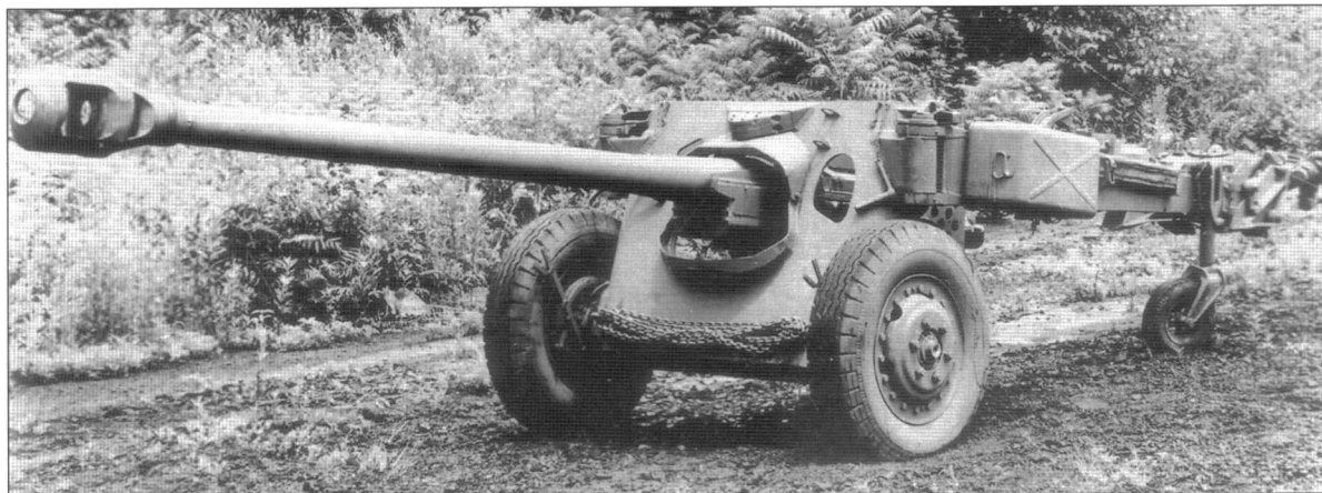
The most radical of the 90mm anti-tank gun designs was the 90mm T13 gun on the T9 carriage. As can be seen here, the shield was used as the central structure of the gun with the trails attached to the top corner. For towing, the trails were folded forward, enveloping the gun in order to reduce the length of the gun in transit. (NARA)
