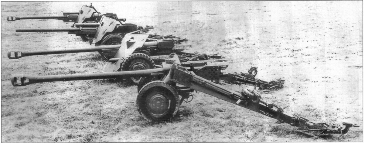
Four different 90mm guns were in development in 1945, although only one entered series production. From front to back these are the 90mm T13 gun on T9E1 carriage; 90mm T20E1 gun on T15 carriage, 90mm T8 gun on T5E2 carriage and 90mm T20 gun on T14 carriage. (NARA)
