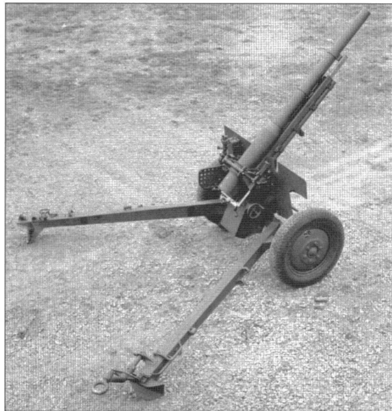
In 1940 the Artillery wanted an expedient anti-tank gun to make up for the lack of suitable modern weapons in the US arsenal. The World War I French M1897 75mm gun was mounted on the M2A3 carriage with direct sights in order to fulfill this role, and over 900 were converted. (USAOM)
