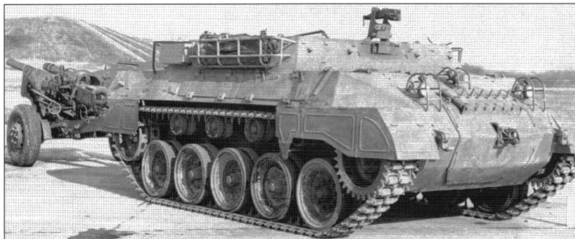
Tank destroyer battalions were authorized to deploy the new M39 armored utility vehicle as the prime mover for the 3in anti-tank gun in September 1944. However, the M39 did not begin to arrive in Europe until April 1945, by which time most of the towed battalions had been converted to self-propelled battalions. (Patton Museum)
