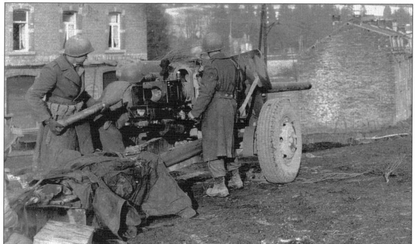
A 3in gun defends a roadblock near Vielsalm, Belgium, on December 23, 1944 during the 7th Armored Division's attempt to withdraw out of the St. Vith salient. It is obvious that the gun has been hastily emplaced as the wheel segments, used to steady the carriage, have not been locked down. (NARA)
