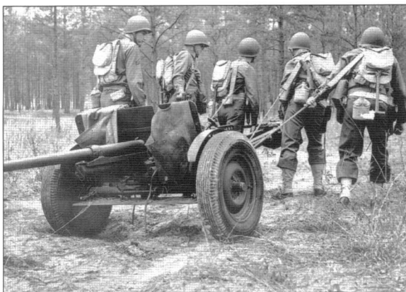
The Infantry Board was not interested in larger anti-tank guns, due to concerns that they could not be handled easily by a four-man crew in combat. This training exercise at the infantry school at Ft Benning in April 1942 shows the prescribed method for towing the 37mm gun by hand. (NARA)
