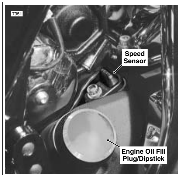
Figure 4-36. Vehicle Speed Sensor Location
