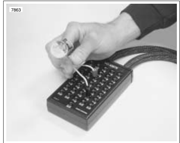
Figure 4-31. Ignition Coil Circuit Test
