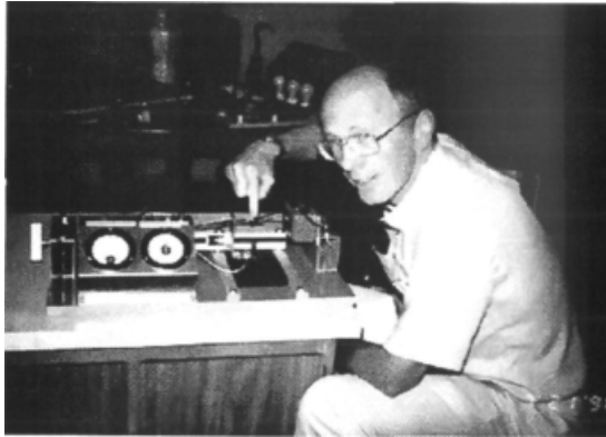
Figure 6-9 Test engineer Rosenthal points to a magnetic field strength mapping device he built for Sweet.
