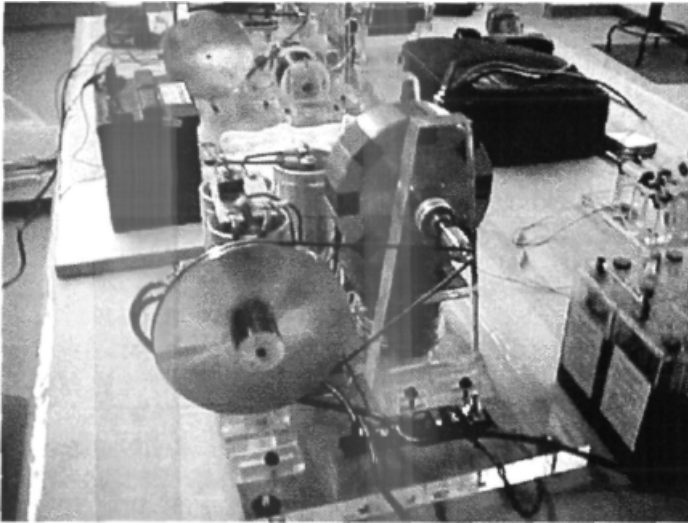
Figure 5-12 Modern Bedini motor prototype which operates off a single battery, powering the load and recharging the battery also.
