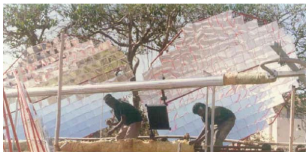
FIGURE 21 A typical configuration of a Scheffler community cooker.
