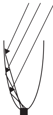
FIGURE 4 A nonimaging concentrator concentrates solar radiation without the need to track the sun.
