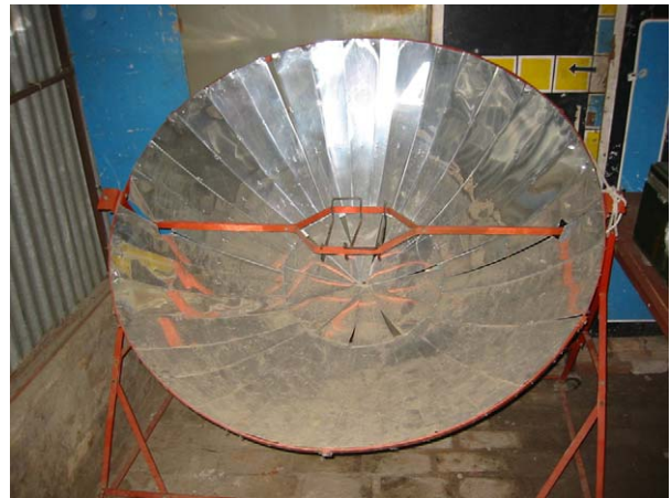
FIGURE 5 Deep parabolic cooker.
