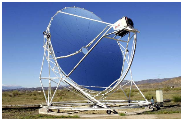
FIGURE 11 Paraboloidal dish solar concentrator with a receiver-mounted Stirling engine operating in southern Spain. Source: Schlaich, Bergemann, and Partner.
